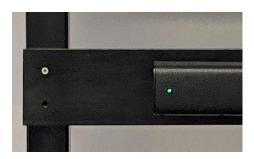
After you turn the power on, a small red light will appear briefly on the left side front of the soundbar. After a few seconds a green light will appear as shown at left. The green light will turn off after about 10 seconds, but the power remains on.
